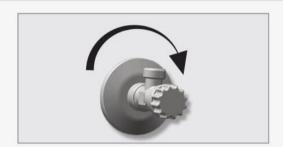
connected to the mains water supply. Use sealing thread or teflon tape to seal the screw thread connection. Fit the wall rosette between the inlet opening of the regulating valve and the surface of the wall.
